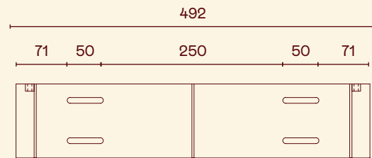
Back fixing placement Featuring slotted holes for ease of installation
